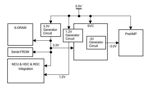
Figure 4.1 Power supply configuration
